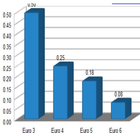
Fig. 1 NOx emission limit for diesel cars (g / km)
