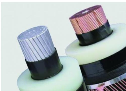
Fig. 15 cables of very high voltage with insulation of crosslinked polyethylene (XLPE) capable to transport currents of the high and very high voltage, with a rated voltage of up to 500kV
